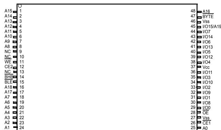
Figure 3. 48-Pin TSOP I (512K x 16/1M x 8) (Top View) [2, 4]
